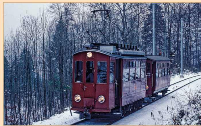
Be 2/2 No.22 + B2 No.224, between Berghof and Uitikon-Waldegg on 2 December 1978. The asymmetrically arranged pantograph is clearly visible. The catenary of the Uetlibergbahn is laterally offset, because between Zürich Selnau/Hauptbahnhof and Giesshübel both direct current operated Uetliberg Railway trains and alternating current operated Sihl Valley Railway trains operate on the same track.
