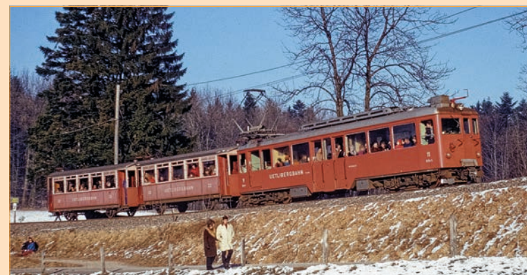
A relief train, encountered at Ringlikon on 31 December 1972. The motor coach BDe 4/4 No.11 (1939) is on its way with the two two-axle coaches B2 No.22 and No.21. The windows of these coaches could be removed. During the summer they were used as open-air observation cars.
